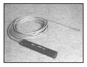
The **MGC-1** also includes a calibration winding that can be used to verify performance or perform a health check.
